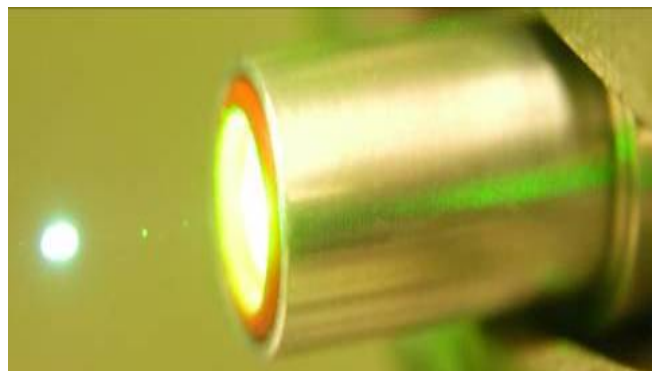
Laser spark formation via a hollow core fiber.
