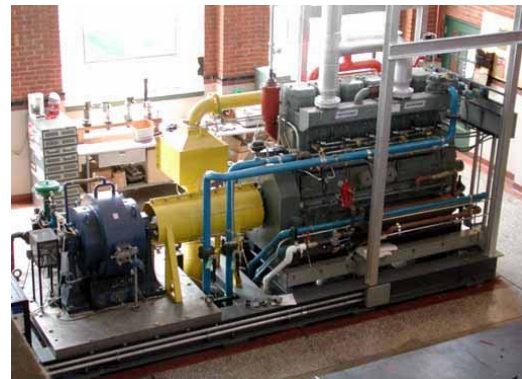
4-Stroke Rich Burn Gas Engine Superior 6G-825
