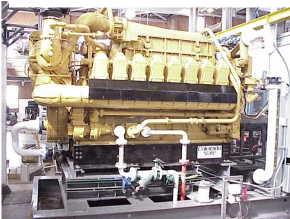
4-Stroke Lean Burn High BMEP Gas Engine – Caterpillar G3516C
