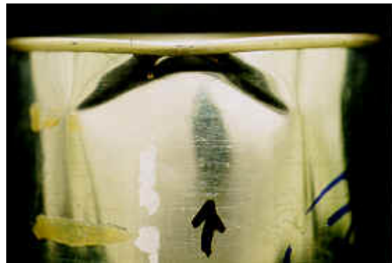
Lower limit of a serious body dent. Body dent is sharp and deep and the double seam has been pulled down below the level of the countersink depth of the can.
