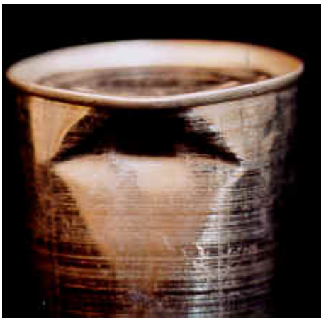
Lower limit of a serious body dent. Body dent is sharp and deep and the double seam has been pulled down below the level of the countersink depth of the can.
